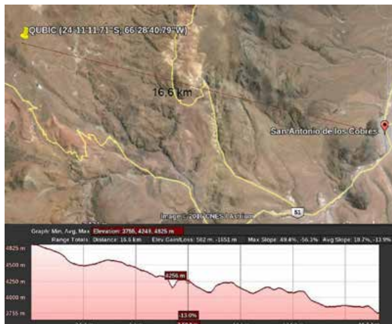
Figure 6. Qubic Site (top) and elevation profile (bottom). The positions of QUBIC and San Antonio de los Cobres are detailed as well as the distance between the sites. The elevation profile is such that it is possible to establish a direct link for communications.
